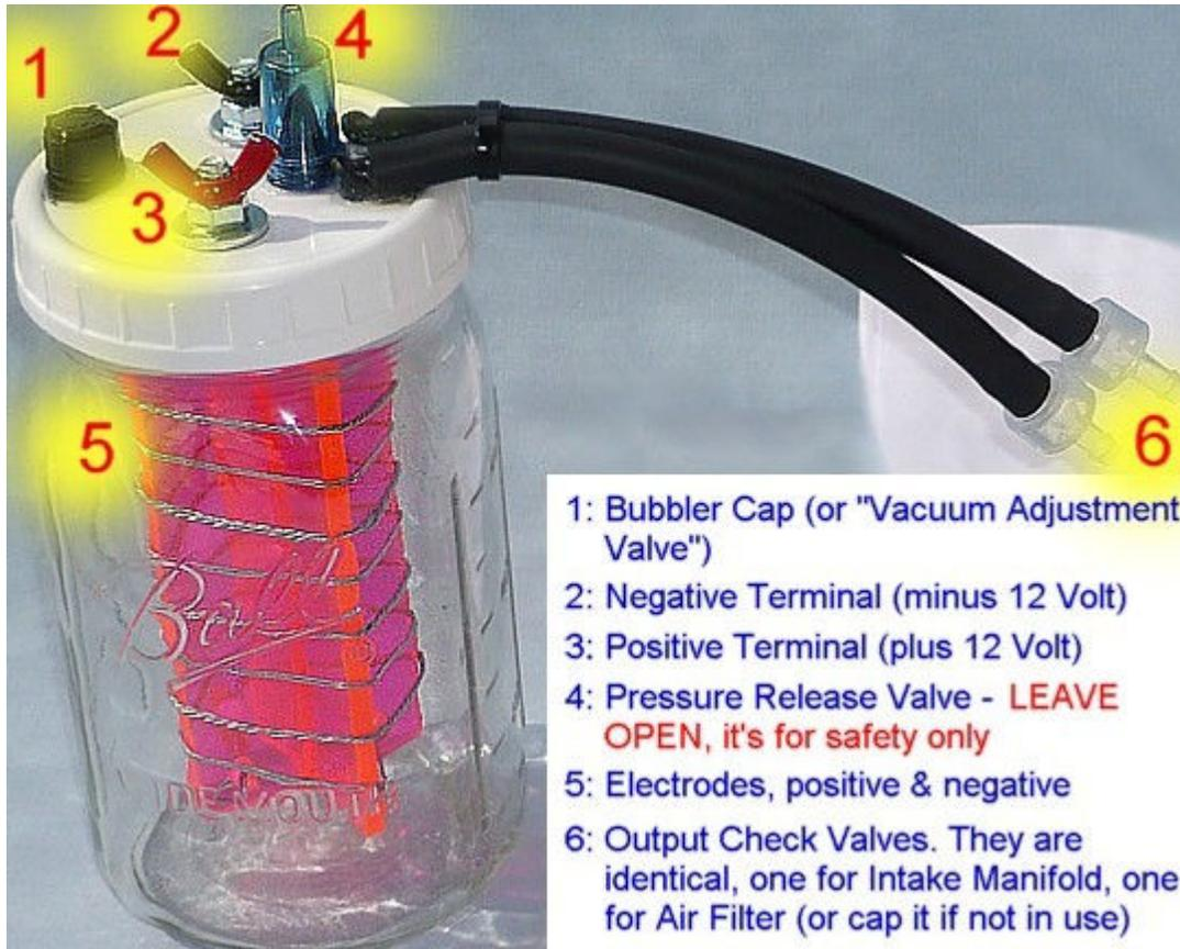
Many readers have asked me about Part 4, the **Pressure Release Valve**; seemingly it is the most misunderstood part - so let me explain a bit more. It is there for safety reasons only. In normal operation, it is dormant, inactive. This is a "check valve", meaning it will allow air/liquid flow in one direction only. In our application, we glue it on top of the device **POINTING UPWARD**. It will let air flow **OUT** but not in. Why?
