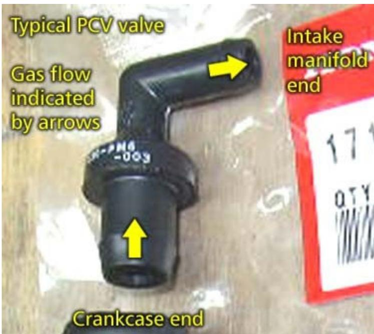
Connect the vacuum line from the device, to a vacuum line that runs to the intake manifold. Make the connection as close as possible to the intake manifold. If the vehicle has a carburetor, make the connection at or below the base of the carburetor. Frequently in older vehicles, there are spare ports available for this purpose. The PCV valve\* line usually makes a good connection. Vehicles with EFI (Electronic Fuel Injection) should also be connected at or near the intake manifold.
